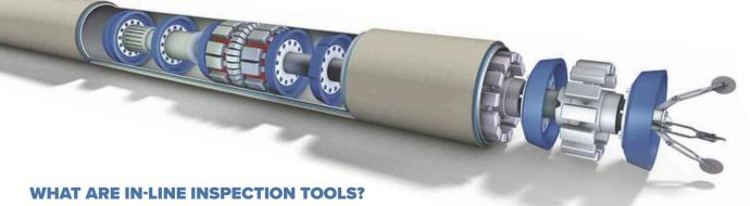
In-line inspection tools, or "Smart Pigs," are electronic tools that travel through pipelines using magnetic sensors to detect irregularities that may indicate corrosion, gouges, cracks or other defects. Using the Smart Pigs, we can identify anomalies and perform preventative maintenance before an incident occurs, making the tools an invaluable asset to our safety program. This proactive measure greatly reduces the probability of a reactive response.
